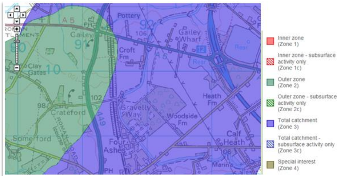
Figure 4-5: Groundwater source protection zones (Environment Agency)
